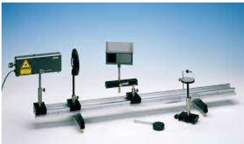
Figure 3: The experimental set up for producing interference with the Fresnel mirror [16]
